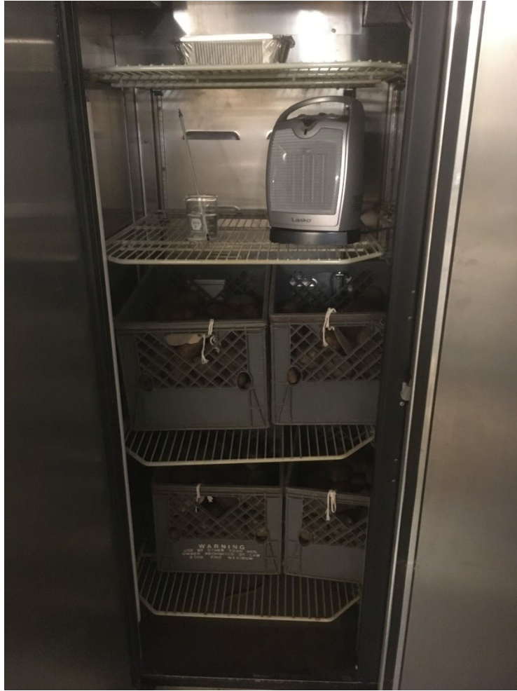
Figure 1. Inside view of the 22°C incubator used for seed aging treatment #3 and #6. The 22°C temperature set-point was maintained with small room heater placed inside the incubator (top shelf). Similar storage conditions were achieved for a separate 32°C incubator (aging treatment #4 and #7 (not shown)).
