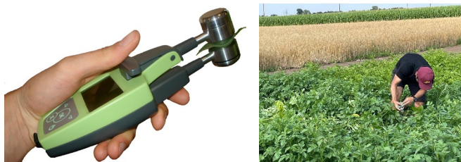
Fig. 1. The Dualex leaf fluorescence sensor (left) and field data collection (right).
